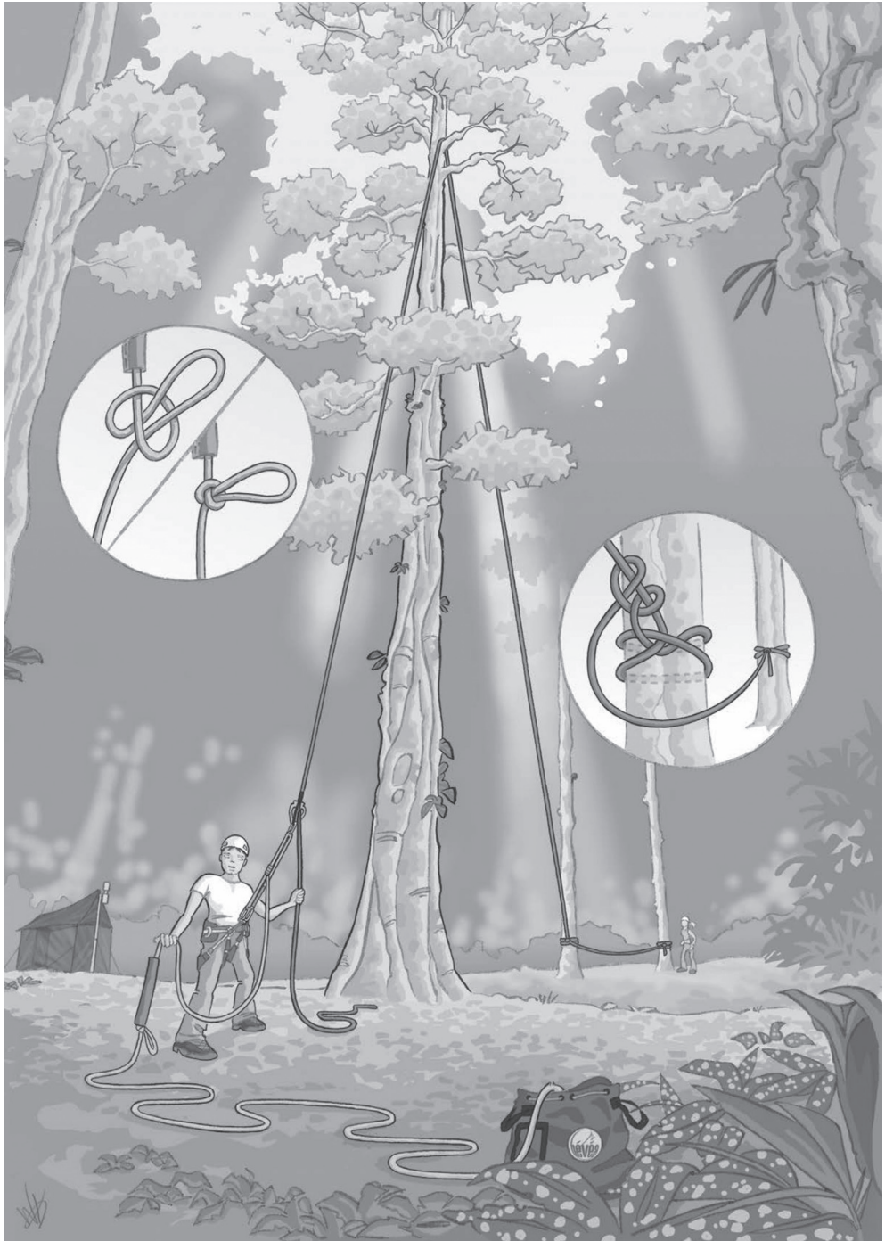
FIG. 1. General view of the system. The static rope is anchored on the tree; the climbing rope is lying on the soil.
