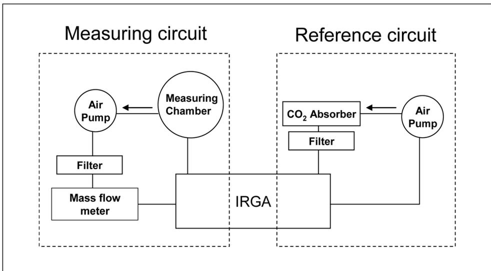
FIG. 1. Scheme of the pneumatic connections in the device to measure the respiration of small soil invertebrates.
